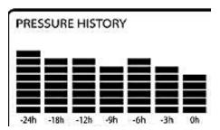
The vertical bars are plotted at each of the seven steps and give the trend over the recorded period. The 0 hour vertical bar will always display at the midline height to indicate the current air pressure. The varying height of bars in other columns on the graph indicates a relative change in air pressure up or down from the 0 hour.
